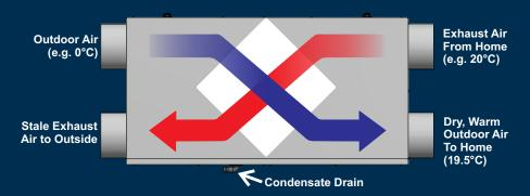
Stale, humid indoor air is continuously exhausted and replaced with 100% outdoor air. Up to 80-95% (depending on model & conditions) of available waste heat from the exhaust air stream is "captured" by the Aluminium Heat Exchanger and transferred to warm the incoming cold outdoor air.
